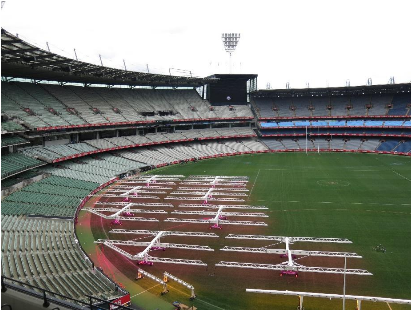
These banks of lights help the grass on the MCG's northern side to keep growing during Melbourne's winter months.
